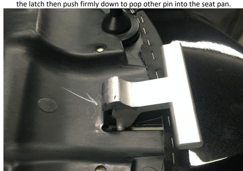
6. To install the seat back on the atv you will need to hold the latch in and push firmly down on the seat till it latches.
