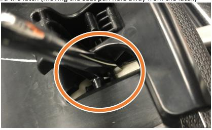
3. While prying on with the screwdriver twisting and pulling on the factory plastic latch to remove the tab/pin on the side you are prying on from the seat pan hole.
